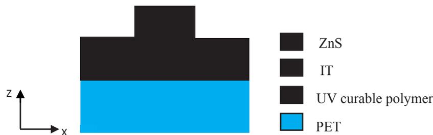
Fig 1. Schematic of the metamaterial unit cell
