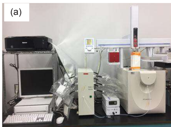
Fig 2 (a). Artificial nose FF-2A for measuring smell.
