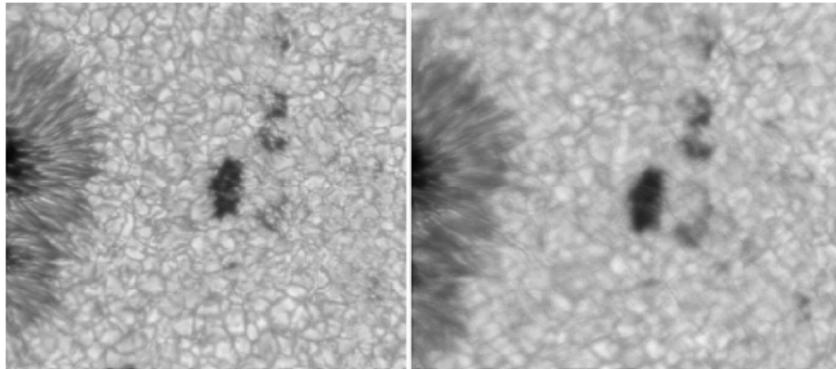
**Fig 8.** The image of an active region with (left) and without (right) AO correction is shown. The field-of-view is  $45 \times 45$  arcsec with a wavelength of 550 nm. The AO was locked onto the dark structure, pore, in the centre of the field-of-view (adapted from [15]).
