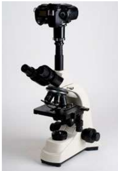
Fig. 1. A camera is inserted in the center tube of a tribocular microscope.
