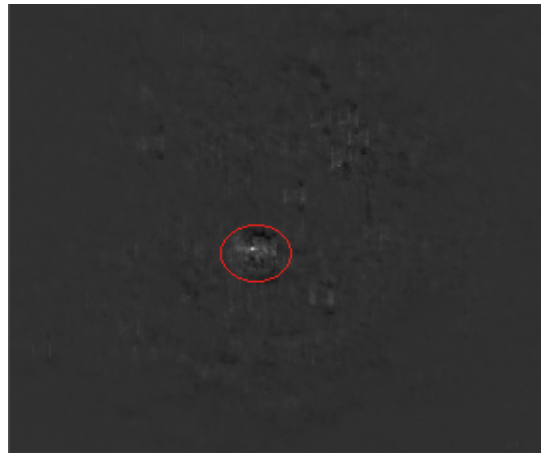
Fig 3. A typical correlation plane obtained by correlating a frame from test video sequence with filter bank of positive and negative filters. The correlation peak is marked by a circle.
