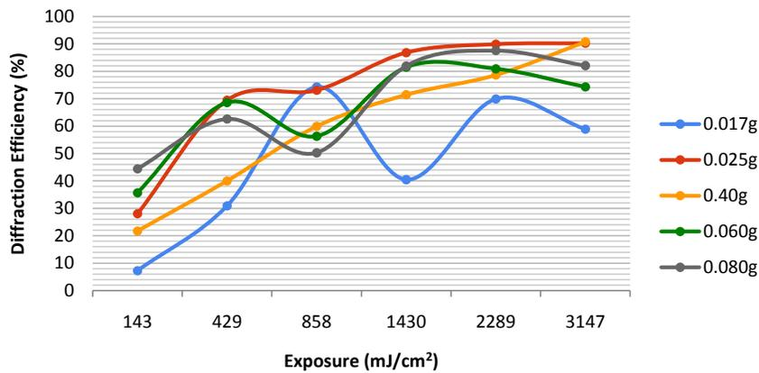
Fig 4. Diffraction Efficiency vs Exposure curves for different dye (EB) Concentrations between 0.017g to 0.080g/100ml de-ionized water.
