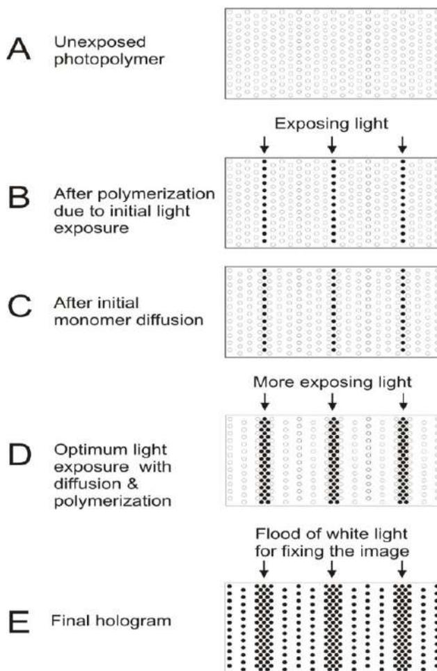
**Fig 1.** Empty circle shows, monomer (s) and filled circle shows polymerized part for (A) Unexposed photopolymer, (B) After initial exposure and polymerization, (C) After initial polymerization and initial monomer diffusion, (D) After optimum exposure with monomer diffusion, (E) Final hologram
