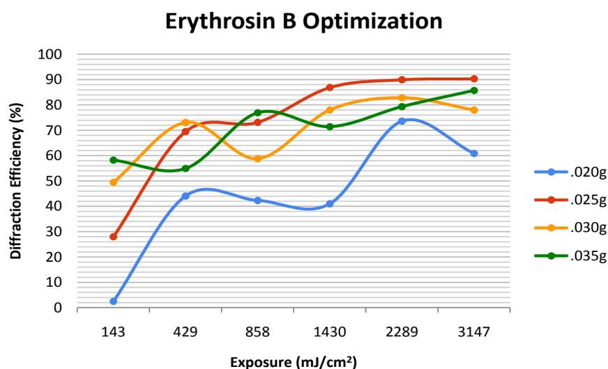
Fig 5. Diffraction Efficiency vs Exposure curves for dye (EB) concentrations of 0.020g, 0.025g, 0.030g, and 0.035g/100ml de-ionized water.
