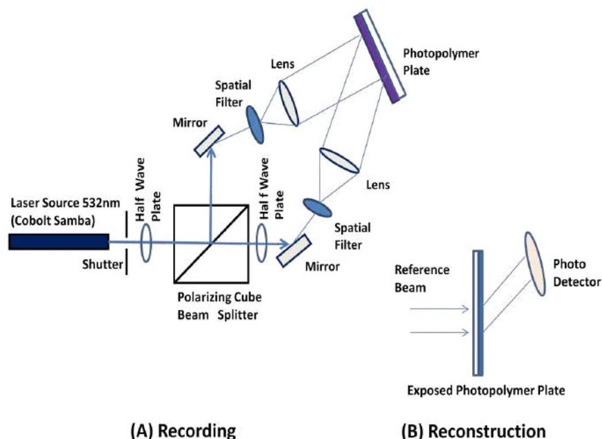
Fig 2. Schematic Diagram of (A) Recording and (B) Reconstruction
