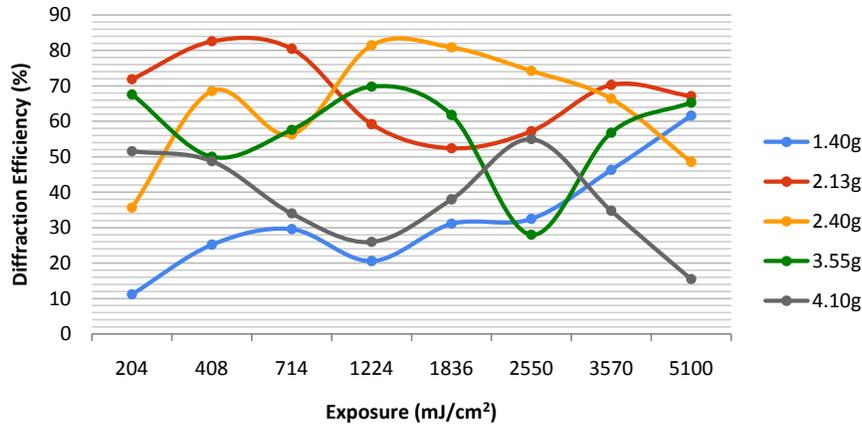
Fig 3. Diffraction Efficiency vs Exposure curves for acrylamide concentrations of 1.40g, 2.13g, 2.40g, 3.55g, and 4.10g/100ml PVA solution
