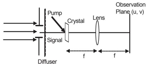
Fig 3. Optical arrangement for dynamic speckle photography
