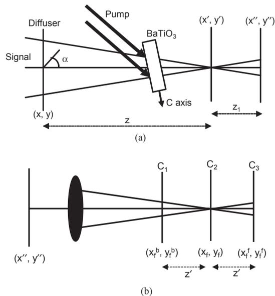
Fig 5. (a) Dynamic speckle recording geometry; (b) Optical correlation using Fourier transform setup
