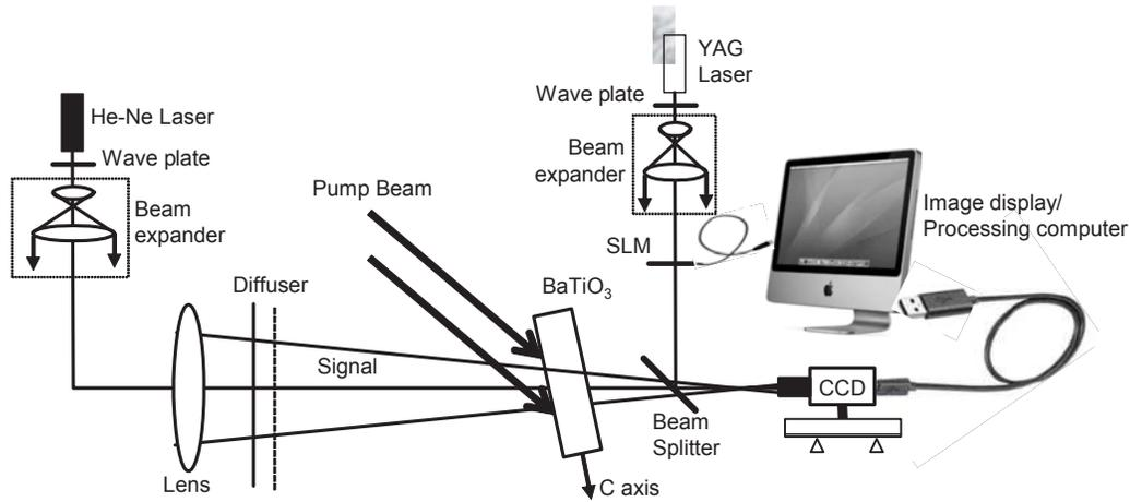
Fig 6. Basic layout of a photorefractive correlator
