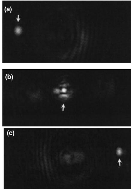
Fig 9. Correlation results obtained for the interference pattern shown in Fig. 8(c) at the observation planes (a) C1; (b) C2; and (c) C3
