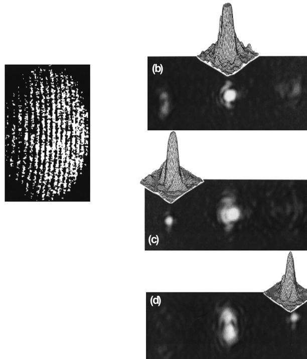
Fig 7. (a) Experimentally obtained double-exposure speckle pattern for a 3-D displacement comprising of  $\varepsilon = 1.0$  mm, and  $\varepsilon \tan \alpha = 200$   $\mu\text{m}$ ; (b-d): correlation outputs : (b) at back focal plane C2 of the FT lens; (c) at plane C1 ( $\sim 7$  cm before C2); and (d) at plane C3 ( $\sim 7$  cm further after C2)
