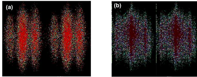
Fig 4. Interference fringes observed in the back focal plane for a 30  $\mu\text{m}$  in-plane object displacement: (a) Double exposure; (b): five exposures
