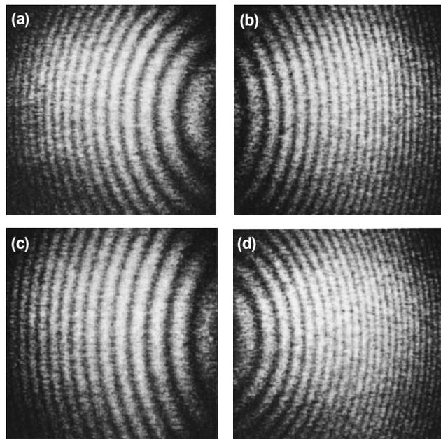
Fig 8. Speckle fringes obtained for a forward object position and tilt angle of (a) 4 mm, 1.58; and (c) 5 mm, 18; and (b) and (d) respective parameters for a backward object position
