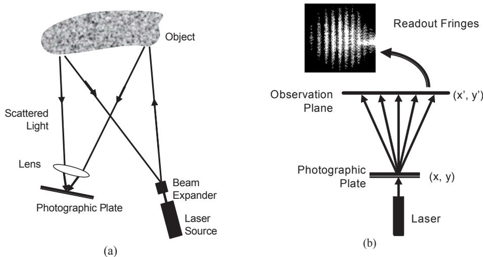
Fig 1. (a) Recording the double-exposure photograph (b) Read-out process to obtain the Young's fringes
