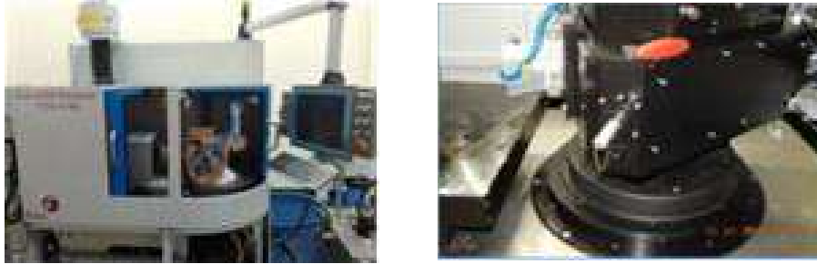
Fig 6. CNC grinding machine and on-machine metrology probe.
