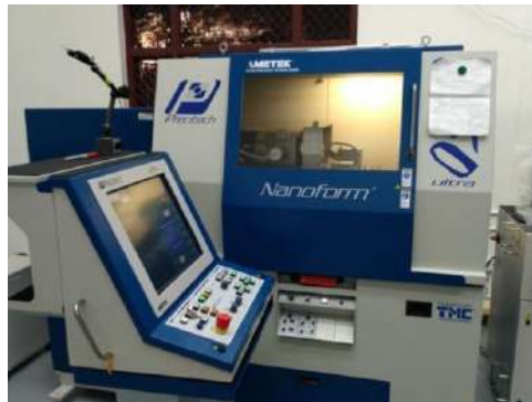
Fig 11. Single Point Diamond Turning Machine -Nanoform 250( M/s Precitech USA) also tested by digital fringe analysis using the Fizeau interferometer or Twyman Green interferometer.
