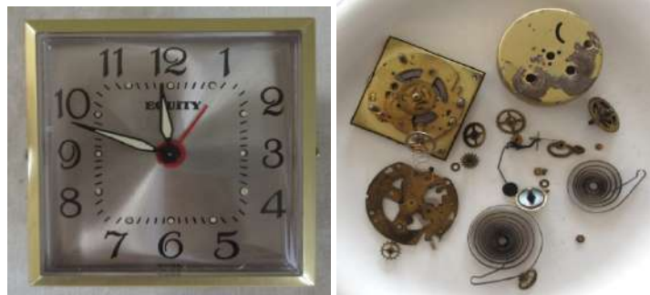
Fig 6. Mechanical clock and its mechanical parts
