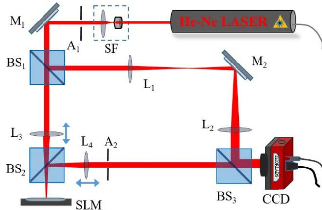
**Fig 1.** Schematic Experimental setup for generation and interferometric analysis of off-axis vortex beam. SF: spatial filter, BS: beam splitter, SLM: spatial light modulator, A: aperture, L: lens, M: mirror, CCD: charge coupled device camera.
