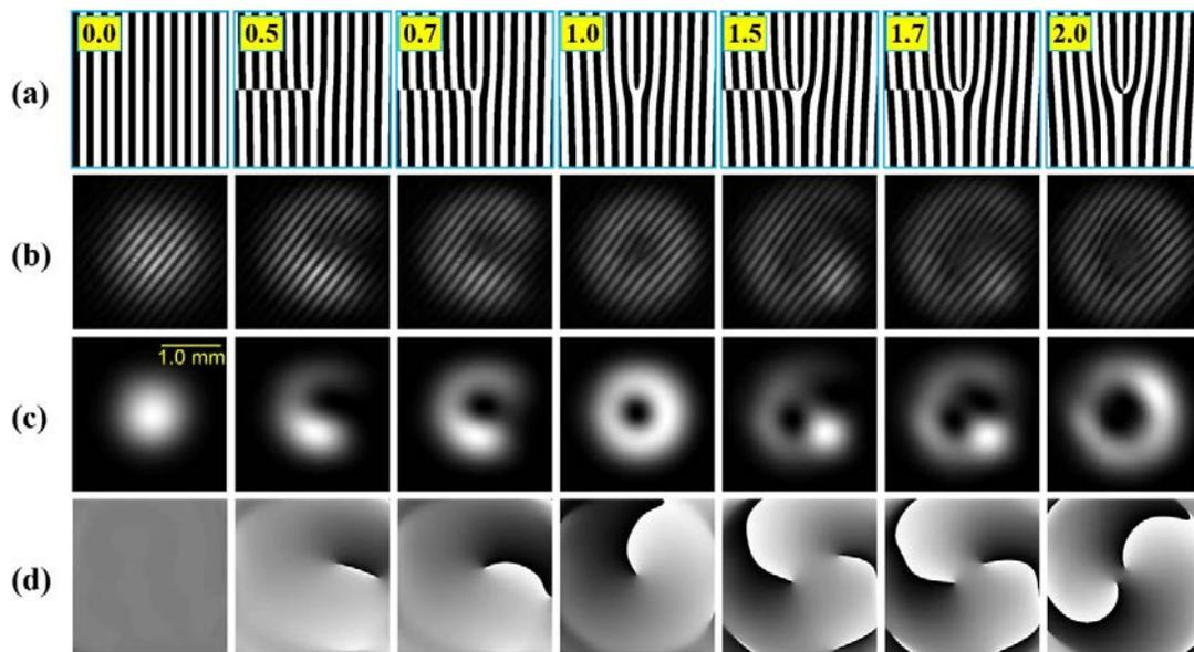
Fig 2. (a) Employed CGH of integer and fractional orders, (b) recorded interferograms, (c) reconstructed intensity and (d) reconstructed phase profile of the integer and fractional order vortex beams.
