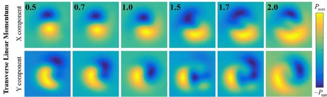
Fig 3. Transverse linear momentum of the vortex beams of different fractional orders.
