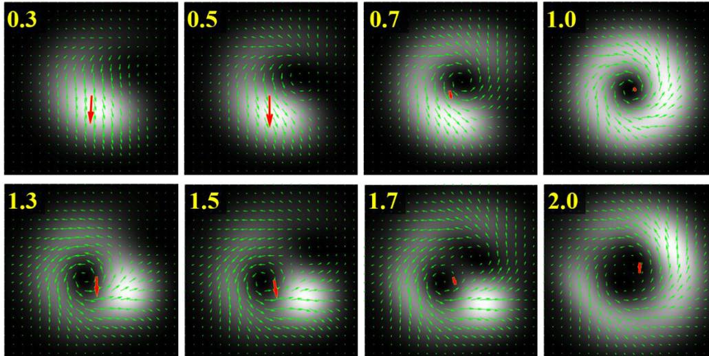
Fig 4. Poynting vector and net transverse linear momentum of the beams with the corresponding intensity profiles in the background.
