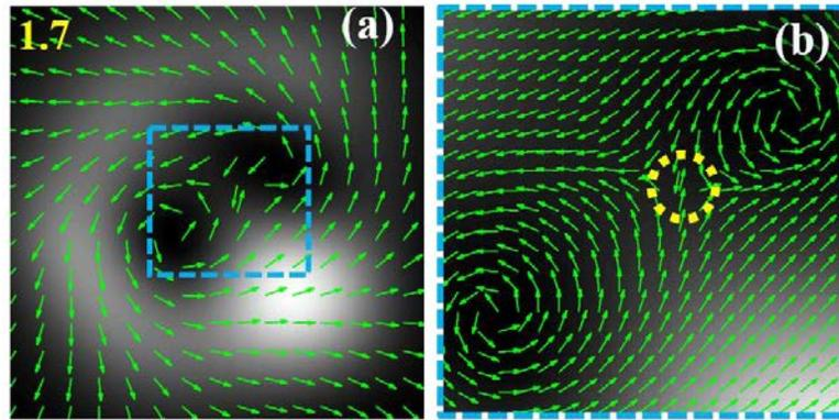
Fig 5. The presence of a saddle point in the Poynting vector distribution corresponding to the field of the OV beam of order 1.7: (a) shows the transverse energy flow where the region in between the point vortices is marked which is magnified and displayed in (b). The position of the saddle point is marked with a yellow dotted circle in (b).
