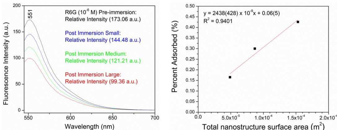
**Fig S3:** (Left) Fluorescence emission spectra of R6G aqueous solution ( $10^{-6}$  M) prior- and post-exposure to the 100 K AgNR substrates of three different dimensions (denoted small, medium and large). (Right) Percent R6G molecules adsorbed onto the 100 K AgNR films versus the total nanostructured surface area of each substrate.
