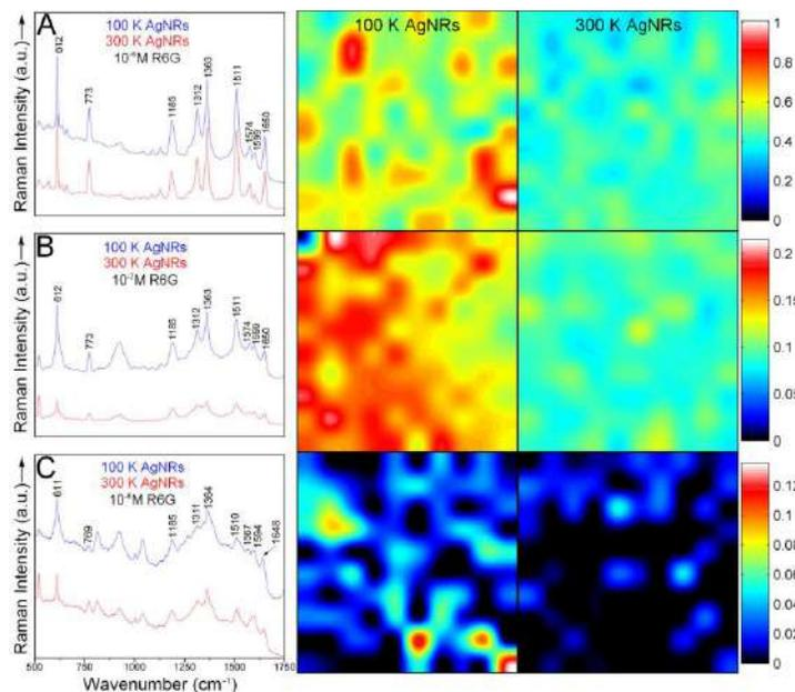
**Fig S2:** (Left column) Average SERS spectra obtained from the adjacent maps. SERS maps constructed from the integrated area of the xanthene breathing mode ( $1625\text{-}1675\text{ cm}^{-1}$ ) of R6G molecules adsorbed on the 100 K AgNR (Center column) and (Right Column) 300 K AgNR (Right column) duplicate samples. Rows A, B, and C designate AgNRs immersed in R6G at  $10^{-6}$ ,  $10^{-7}$ , and  $10^{-8}$  M, respectively.
