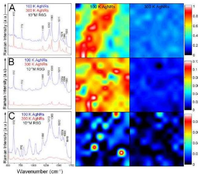
**Fig 2.** (Left column) Average SERS spectra obtained from the adjacent maps. SERS maps constructed from the integrated area of the xanthene breathing mode ( $1625\text{--}1675\text{ cm}^{-1}$ ) of R6G molecules adsorbed on the 100 K AgNRs (Center column) and 300 K AgNRs (Right column). Rows A, B, and C designate AgNRs immersed in R6G at  $10^{-6}$ ,  $10^{-7}$ , and  $10^{-8}$  M, respectively.
