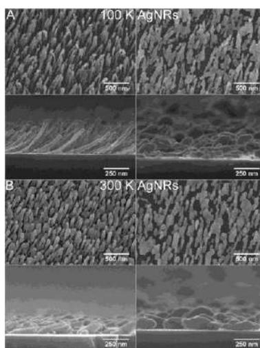
Fig 1. AgNR thin films fabricated at (A) 100 K and (B) 300 K. Top view and cross section SEM images of the AgNR films (Left) prior- and (Right) post-exposure to  $10^{-6}$  M of R6G aqueous solution.
