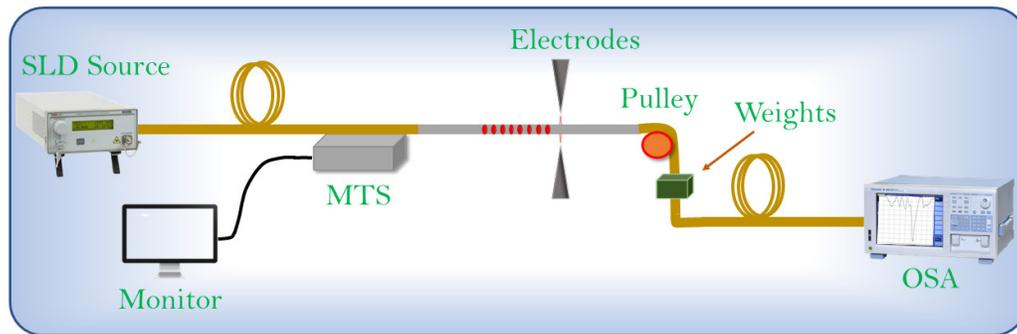
Fig 2. Schematic of the experimental set-up for fabricating the LPG; SLD: Super-Luminescence Diode, MTS: Micro-Translational Stage, OSA: Optical spectrum analyzer;
