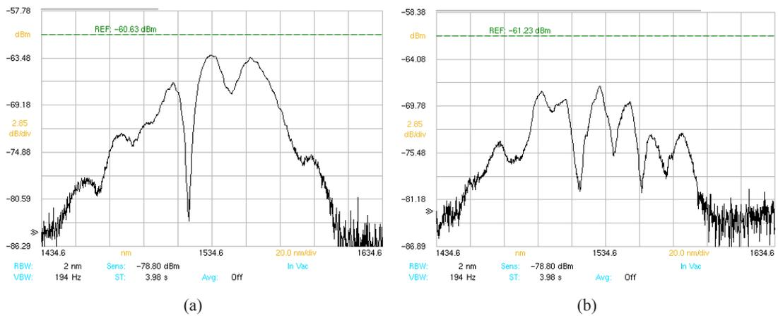
**Fig 4.** Transmission spectra of fabricated LPG on FMF (a) 1310 BHP and (b) 980 HP fiber.
