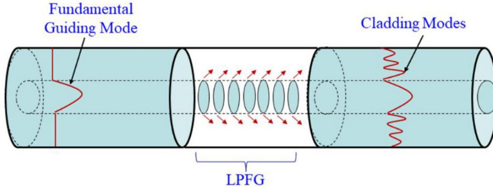
Fig 1. Schematic of the Long period grating
