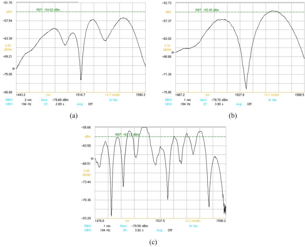
**Fig 3.** Transmission spectra of LPG fabricated SMF 28e+ for (a) arc time=300ms,  $\Lambda = 500\mu\text{m}$ , std power; (b) grating length of 0.5cm; (c)  $LP_{01}$ - $LP_{08}$  modes. Up to eight order modes have been observed at the lowest length of the 5.3 cm of grating length for arc time and periodicity of 300ms and  $450\mu\text{m}$  respectively with standard power.
