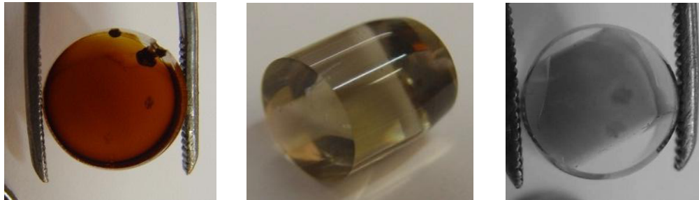
Fig 1. Photographs of composites containing C 60 fullerene (left) and Astralen (middle and right)
