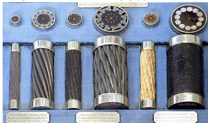
Fig 3. 1858, 1865 and 1866 submarine telegraph cable samples.
