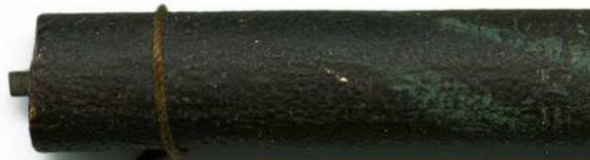
Fig 1. Copper wire covered with Gutta-Percha for insulation, 1850 Dover to Calais cable.
