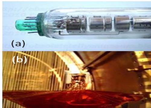
Fig 3. Electron beam source of (a) cathode ray tube (CRT) with (b) grid modifications for pulse biasing the beam extractor.
