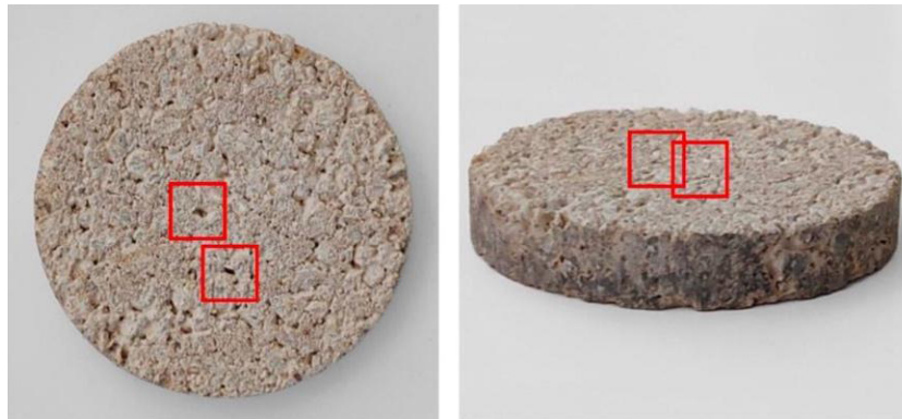
Fig 9. Surface views illustrating the perception of surface cavities under different illumination geometries: top view at normal incidence ( \beta = 0^\circ , left) and side view at grazing incidence ( \beta = 60^\circ , right).
